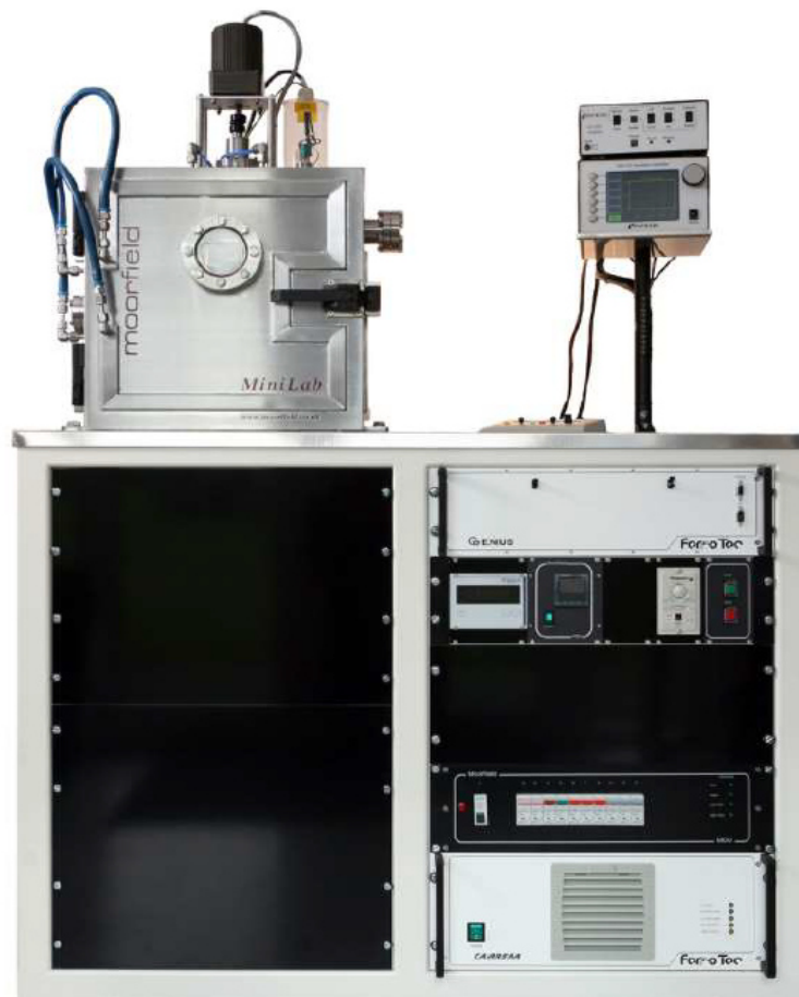
Figure VII.3: The RF sputtering MiniLab 060.
