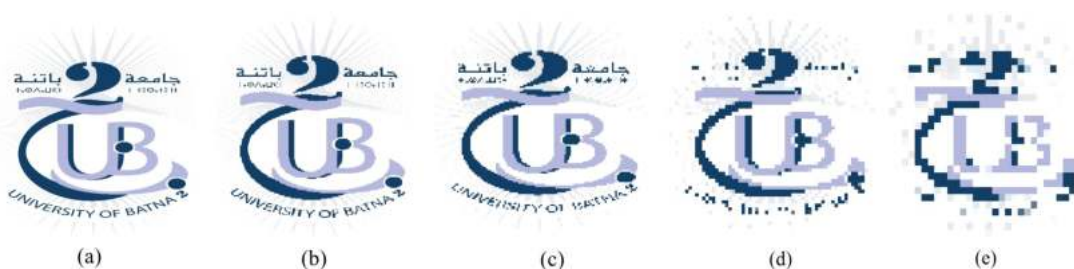
Figure 2.3: Different Pixel Resolutions for logo of university of Batna 2. (a) a block of [512,512] pixels, (b) have a block of [256, 256] pixels, (c) have a block of [128, 128] pixels, (c) have a block of [64, 64] pixels, (e) have a block of [32, 32] pixels.
