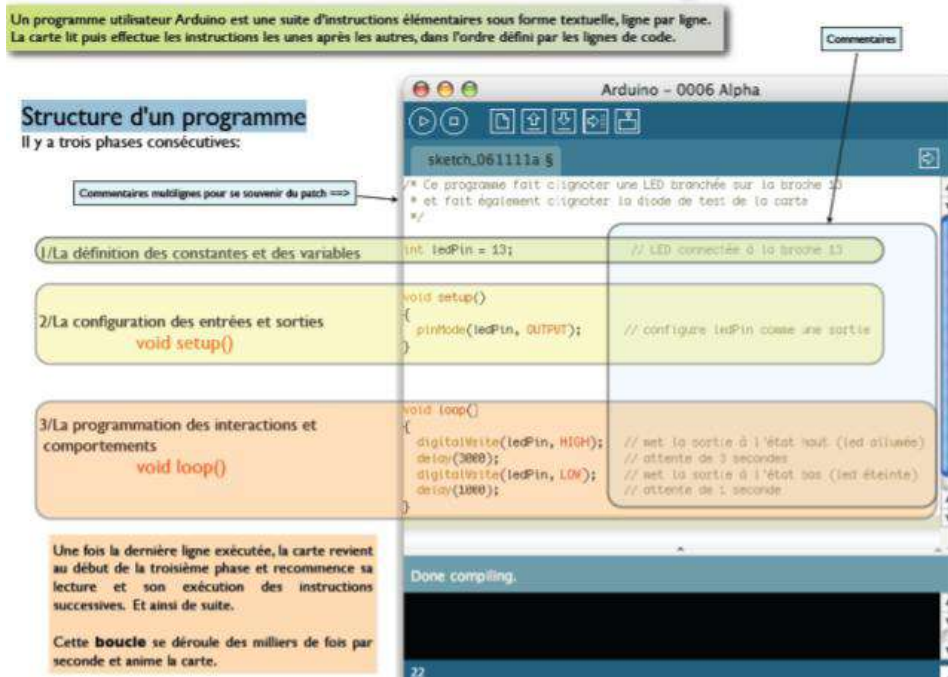
Figure 4.9: Structure d'un programme Arduino [90]
