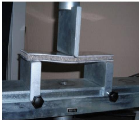
Figure II.15: Three-point bending test configuration according to the ASTM C 393-62 b test specimen under loading [114].
