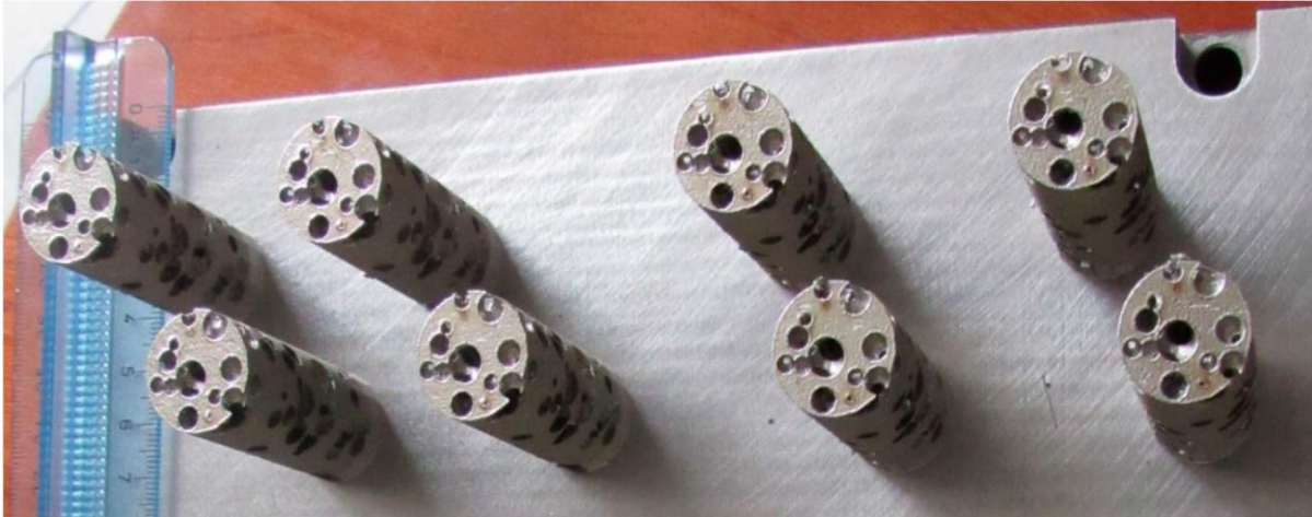
Figure I.18: Cylindrical random foams manufactured by means of LPBF [70].
