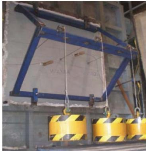
Figure I.42 Configuration du test d'incendie (Guerrieri and Fragomeni 2010) [107]
