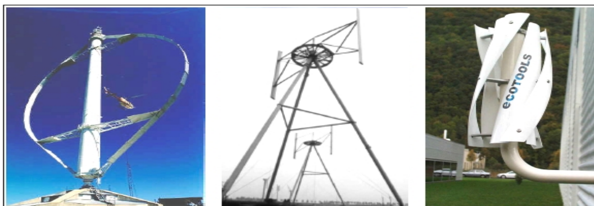
(a) Turbine Darrieus (b) Turbine Darrieus de type H (c) Turbine Savonius
