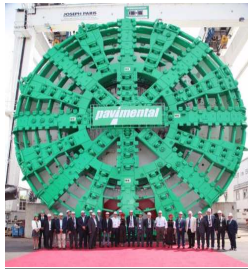
Figure 1.19 Tunnelier géant de Santa Lucia, Italie (TunnelTalk, 2016)
