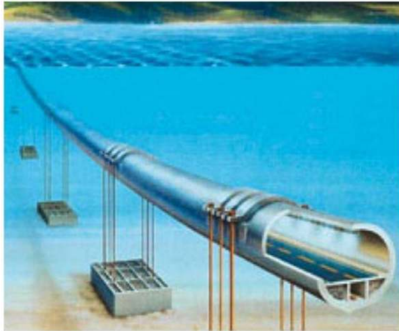
Figure 1.7 Tunnel flottant submergé (Wallis, 2010)
