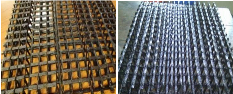
Figure. II.5 Types de géogrilles 3D
