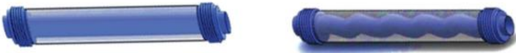
Figure V.2. The geometry of the absorbers, straight (left), and the new S-shaped (right) [10]. To ensure the fidelity of the comparison, the S-shaped absorber is put under the same geometrical characteristics and operating conditions as the straight one, as illustrated in Tables V.1 and V.2.
