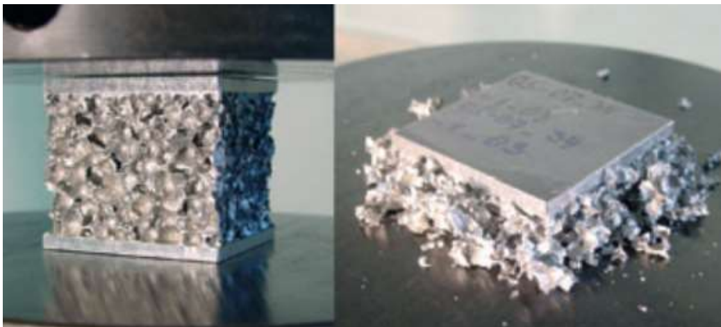
Figure II.2 Before and After Compression Testing: Aluminum Foam Sandwich Specimen with t_s=34\text{mm} Thick Sandwich Core.
