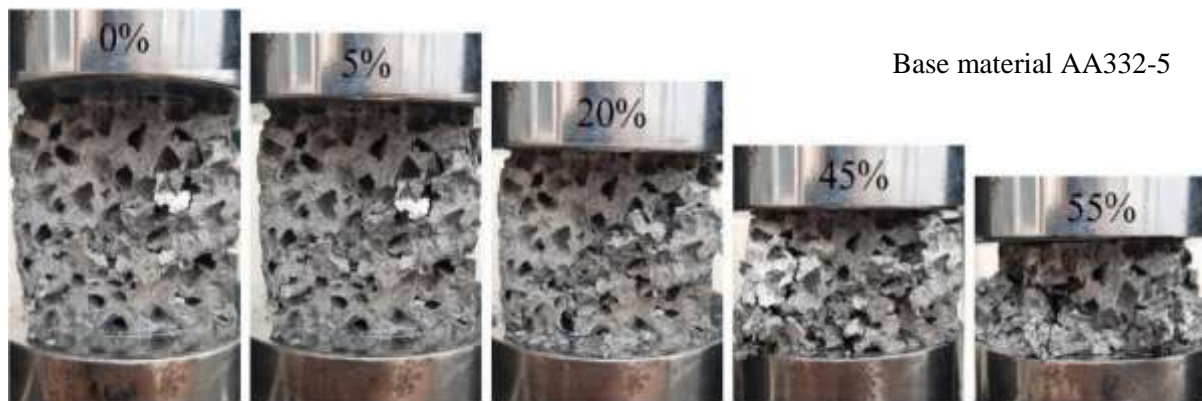
Figure II.11 Deformation mode of aluminum foam specimen under quasi-static compression test.
