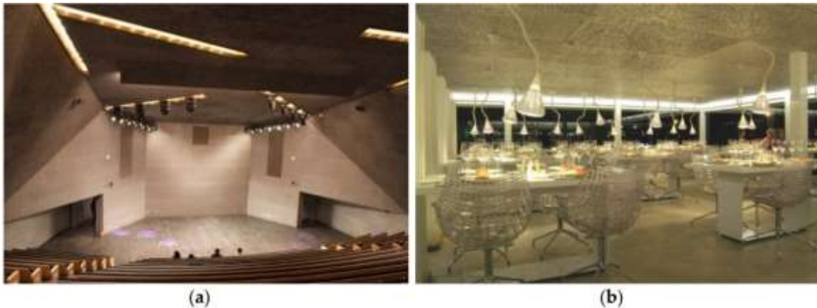
Figure I.18 a) Audience Hall, b) Restaurant covered by Alusion foam for sound control.
