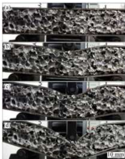
Figure II.25 deformation mode of AFSS under bending test with 3 mm steel panel and 40 mm foam core at different time.
