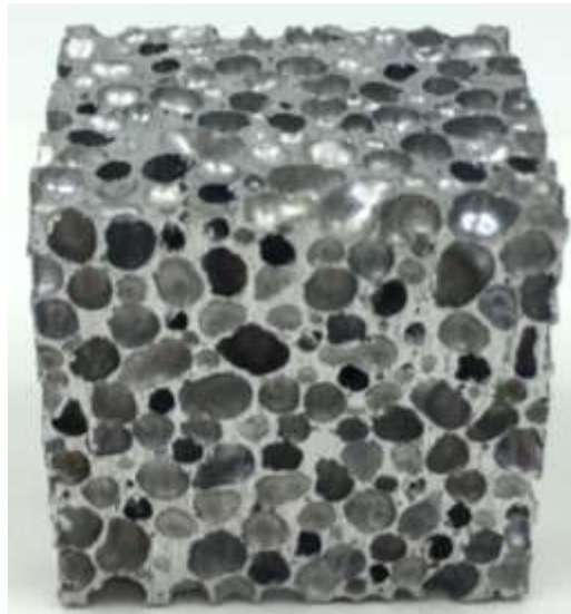
Figure I.2 Closed-Cell Aluminum Foam.
