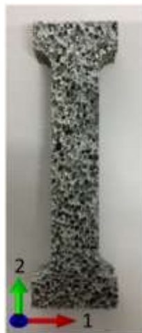
Figure II.34 Specimens for uniaxial tension.
