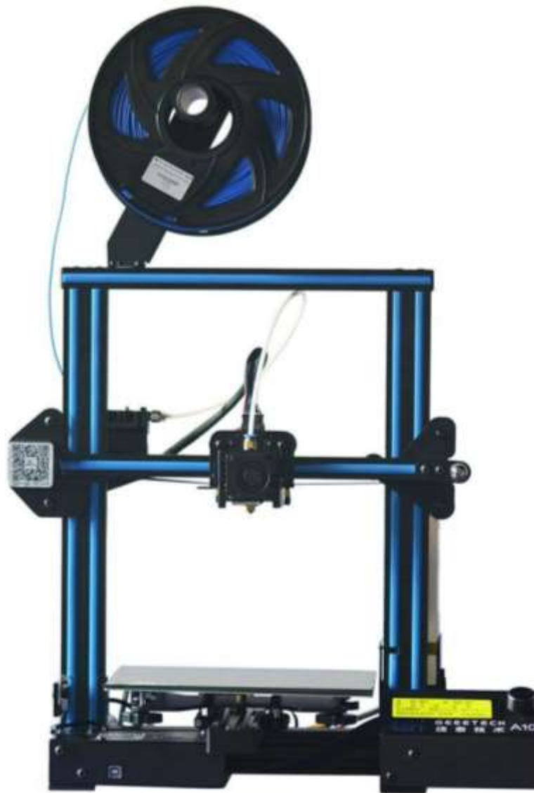
Figure 2: Geetech A10M FDM printer.
