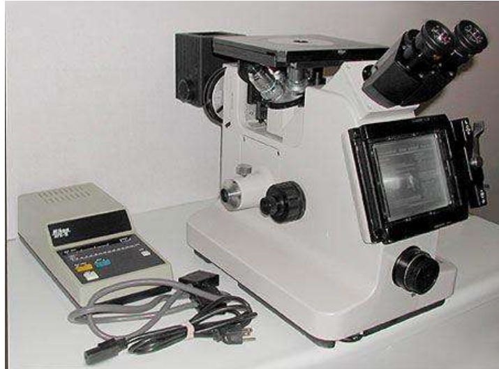
Fig. IV.6 : Microscope, inverted metallograph, objectives: 5X, 10X, 20X, 40X eyepieces: 10X with microflex AFX11 photo system.
