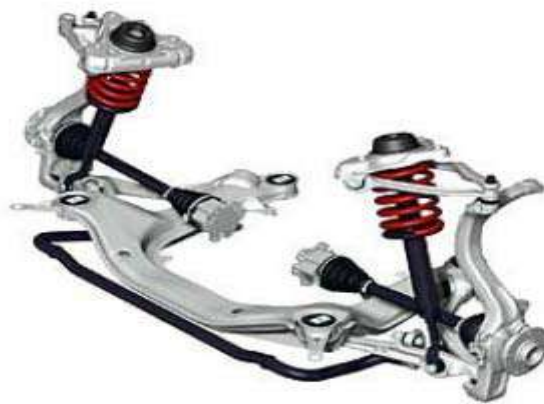
Figure 1. 3 - Suspension de type double triangulation [5]
