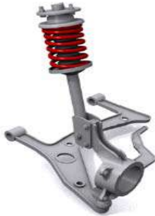
Figure 1.1 - Suspension de type Mc Pherson [5]
