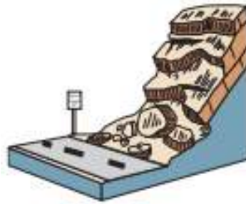
Figure 1-12. Slope movements type: Falls
