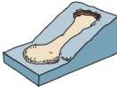
Figure 1-17. Slope movements type: Flows
