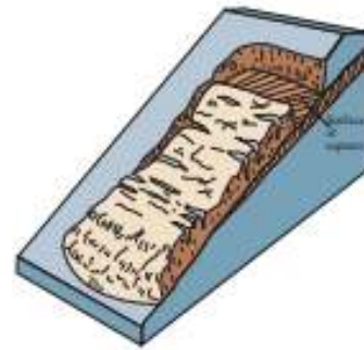
Figure 1-15. Slope movements type: Translational slides
